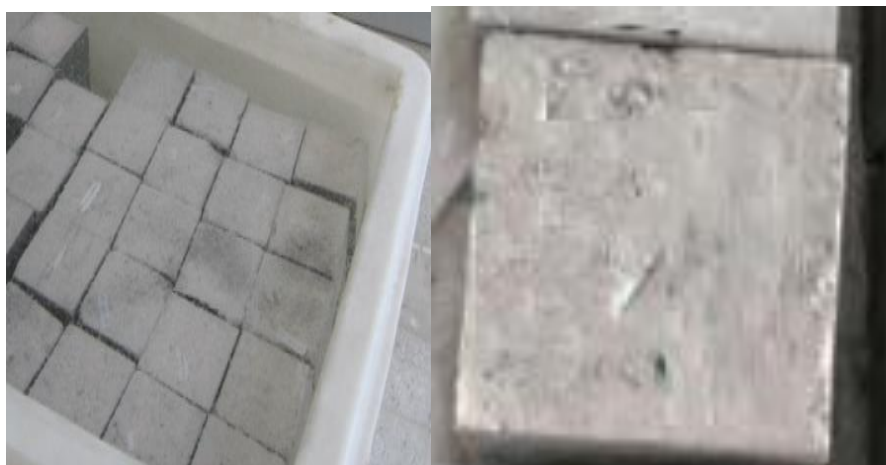
Figure 3. Concrete sample curing pond
