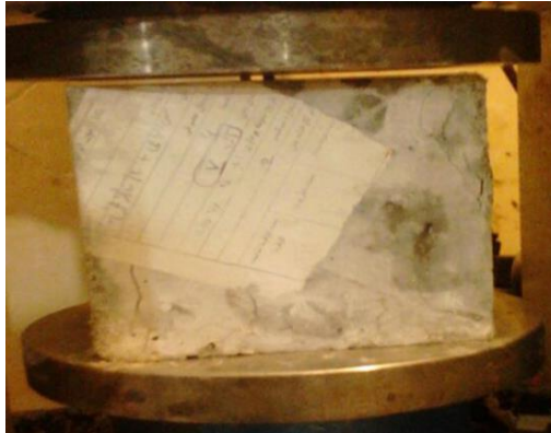
Figure 4. Compressive strength test of geopolymer samples
