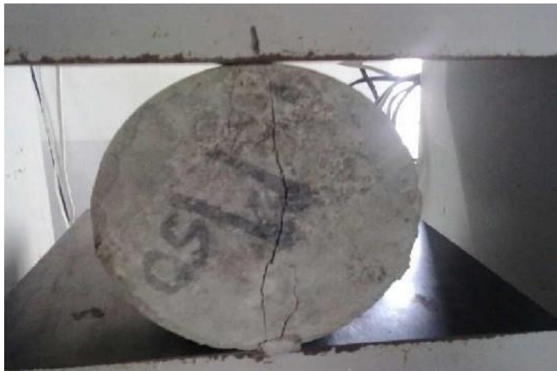
Figure 8. Compressive failure of concrete cylinder
