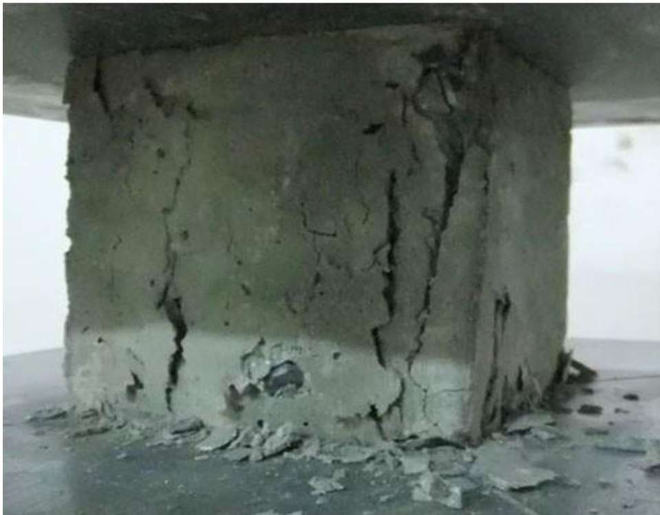
Figure 6. Compressive failure of concrete cube
