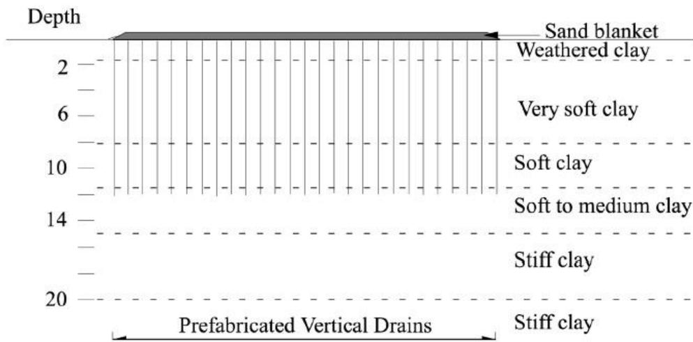
Figure 1. Cross section of an embankment with the subsoil profile, Second Bangkok International Airport, Thailand [30].
