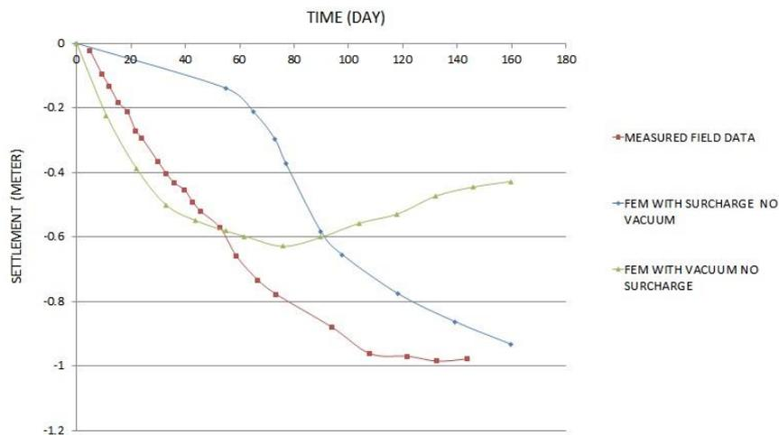
**Figure 6.** Settlement curves of (centerline) (a) FEM modeling in the case of PVDs without any surcharge preloading and (b) FEM modeling in the case of PVDs without any vacuum preloading vs. Field measured data
