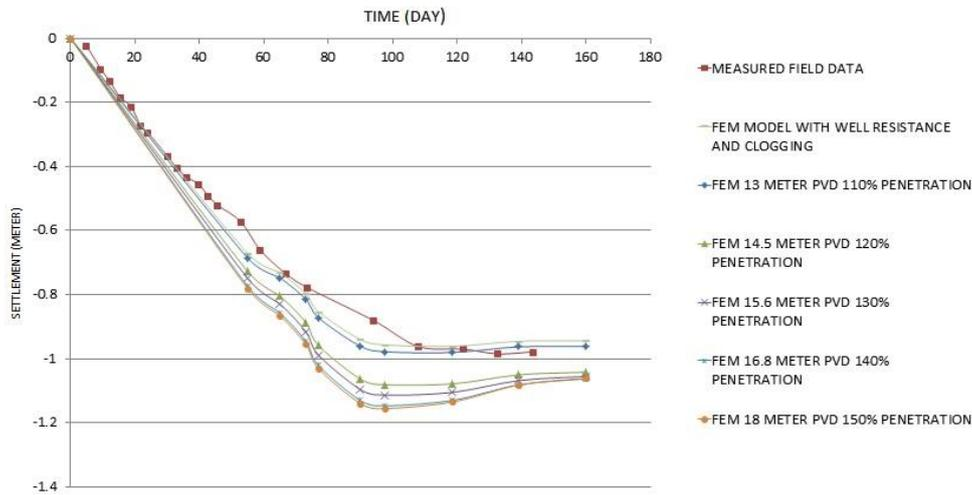
**Figure 8.** Settlement curves of the FEM modeling of TV2 test embankments (centerline) for 110,120,130,140 and 150 percent full penetration corresponding to 13, 14.5, 15.6, 16.8 and 18 meter
