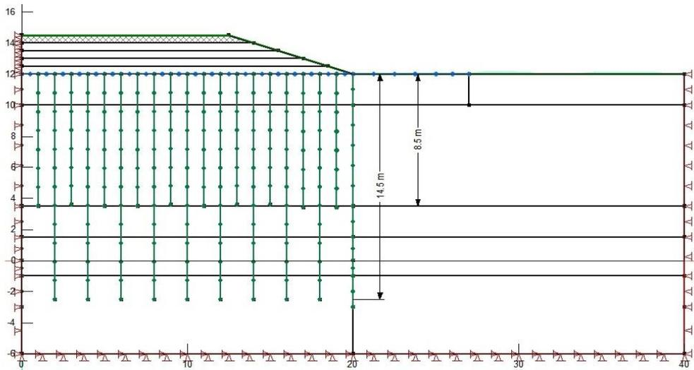
Figure 10. schematic of proposed method "One and Between Configuration"
