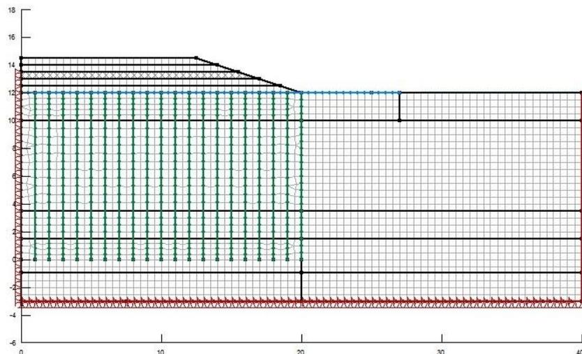
**Figure 4.** geometry and the mesh of finite element of TV2
