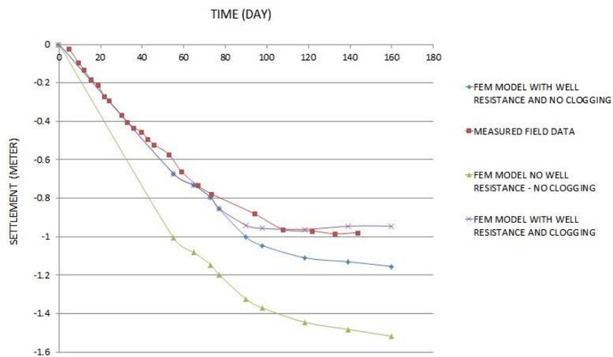
**Figure 5.** Settlement curve of (centerline) (a) FEM model with no well resistance, and no clogging (b) FEM model with well resistance, and no clogging (c) FEM model with both well resistance and clogging vs. Field measured data
