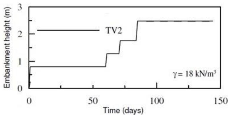
Figure 2. Multi-stage loading for embankments TV2 [31]
