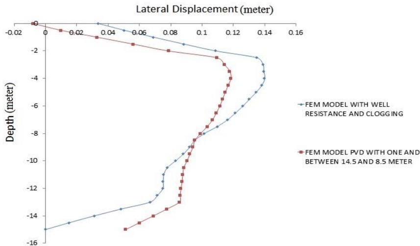
**Figure 12.** Lateral displacement curve (embankment toe) of "One and Between Configuration" in compare to Verified FEM model
