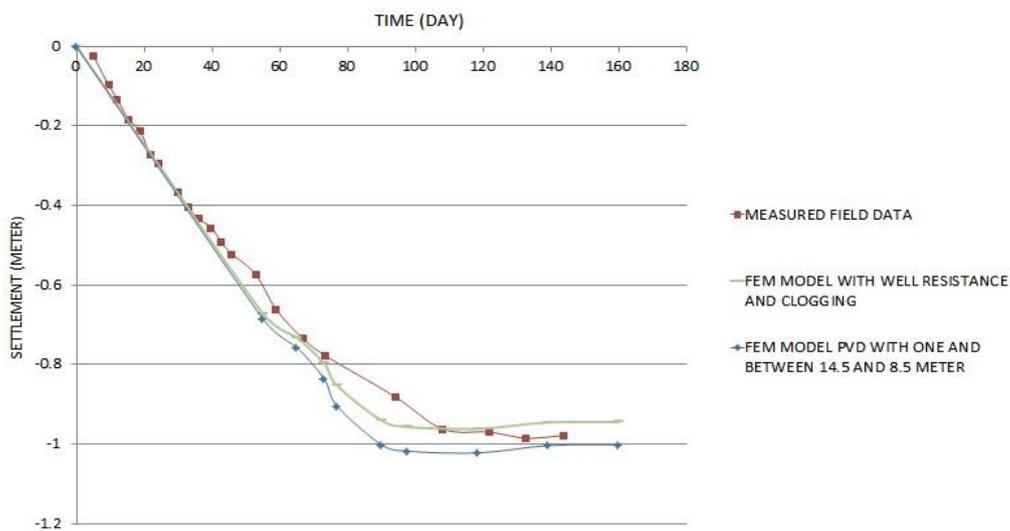
Figure 11. The settlement curve (centerline) of "One and Between Configuration" in compare to field measured data and verified FEM model
