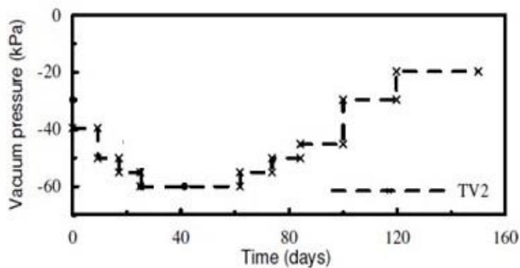
Figure 3. Time dependent vacuum pressure TV2 [31]
