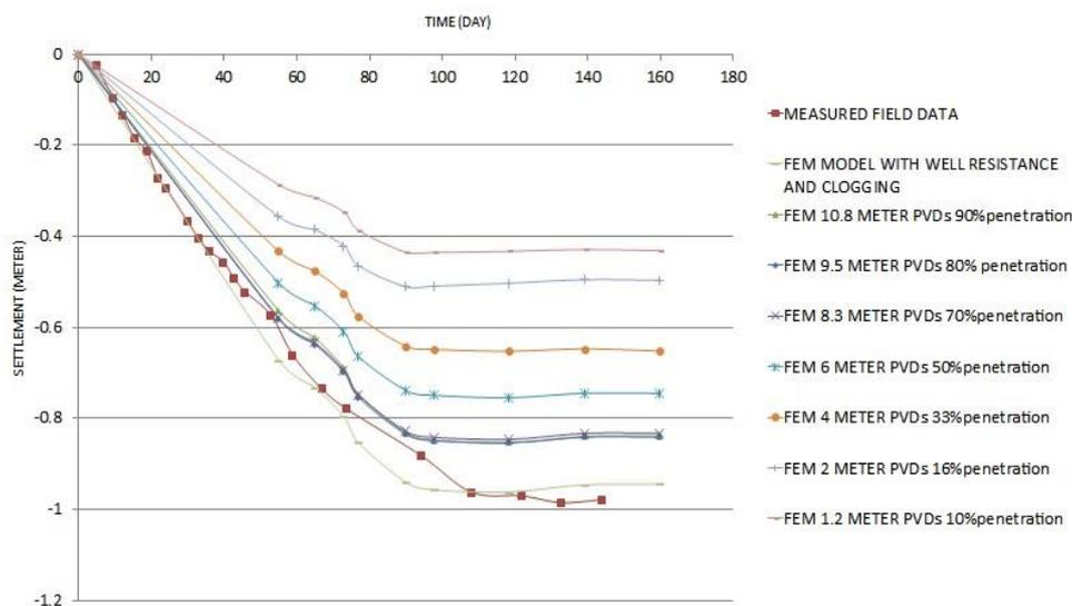
Figure 7. Settlement curves FEM modeling of TV2 test embankments (centerline) for 90,80,70,50,33,16 and 10 percent full penetration corresponding to 10.8,9.5,8.3,6,4,2,1.2 meter
