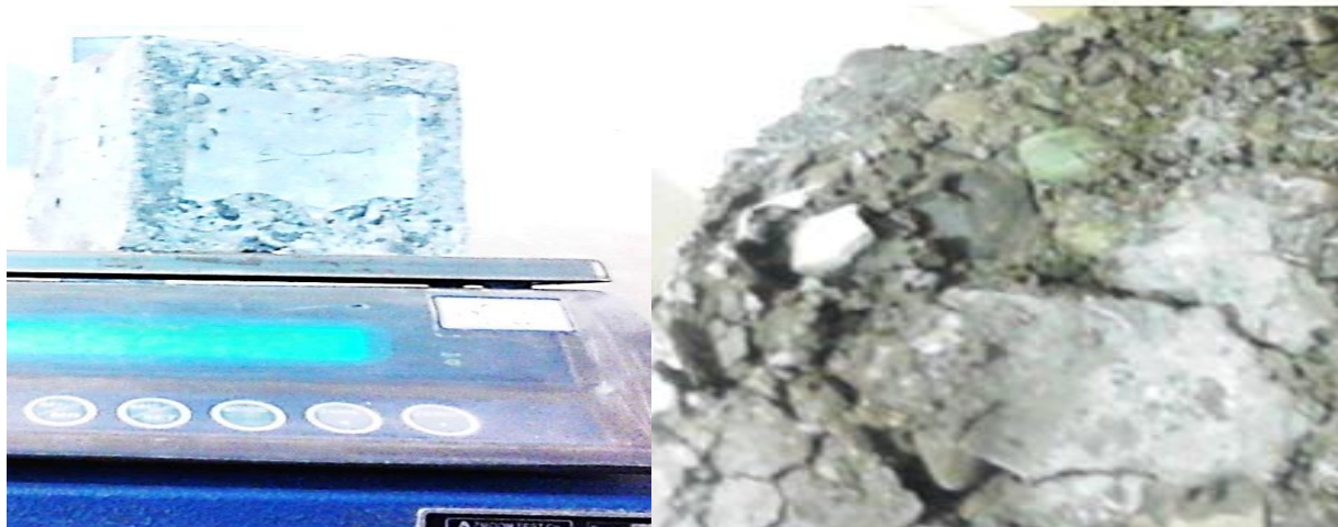
Figure 4. Corrosion on the surface of concrete specimen in the acid environment
