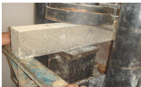
Figure 5. Constructed beam under one-point flexural loading
