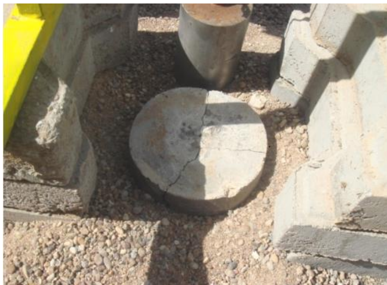
Figure 6. Impact loading test
