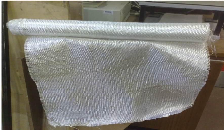
Figure 1. GFRP sheet to strengthen the wall
