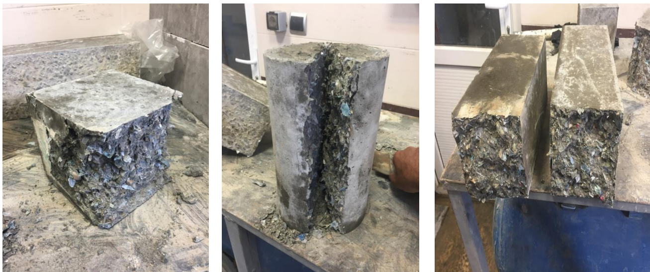
Figure10. Failure mode after mechanical tests
