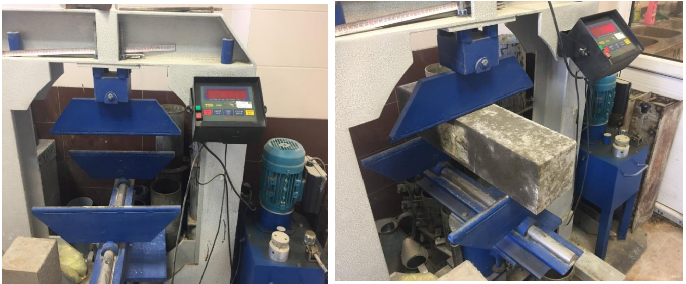
Figure 8. Flexural strength test setup
