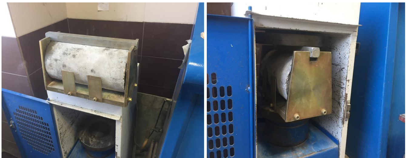
Figure 5. Splitting tensile specimen and test apparatus
