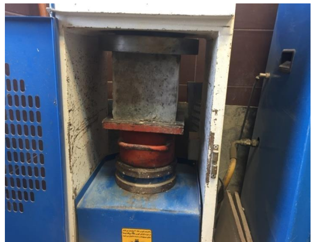
Figure3. Compressive strength specimen and test machine
