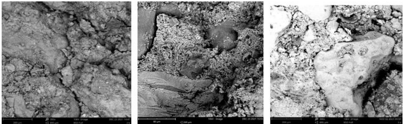
Figure 5(b). SEM for sample S4 at 7, 28 and 56 days respectively
