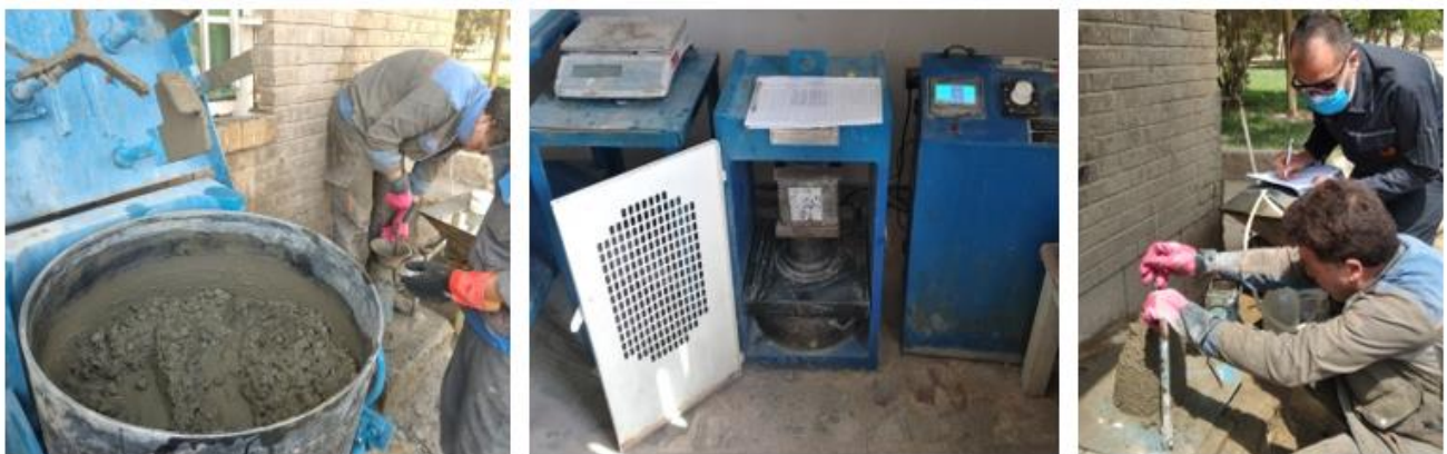
Figure 4. Preparation of concrete mixes and related tests
