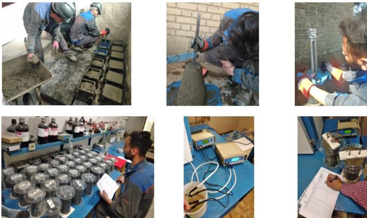
Figure 3. Preparation of concrete mixes and related tests
