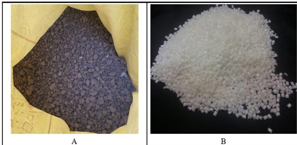
Figure 2. Used recycled materials A: steel slag, B: rPET
