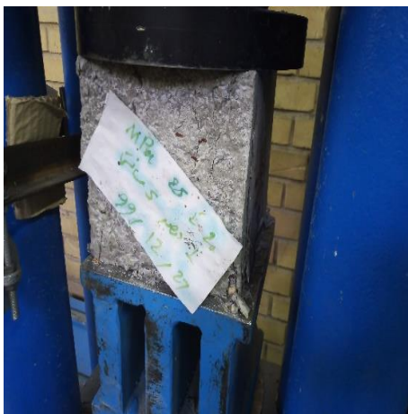
Figure 4(a). The compression strength test of the concrete
