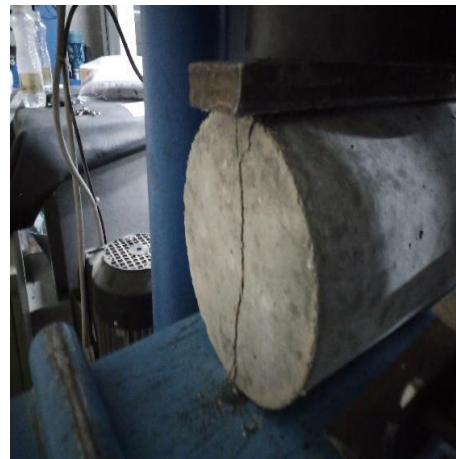
Figure 4(b). The tensile strength test of the concrete
