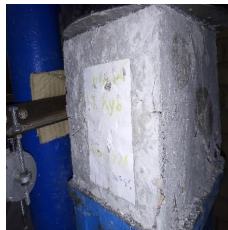
Figure 5. Cubic specimens containing steel fibers after breaking
