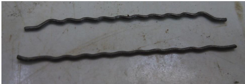
Figure 8. Fibers in the initial state (top) and fibers after extraction from concrete (bottom)
