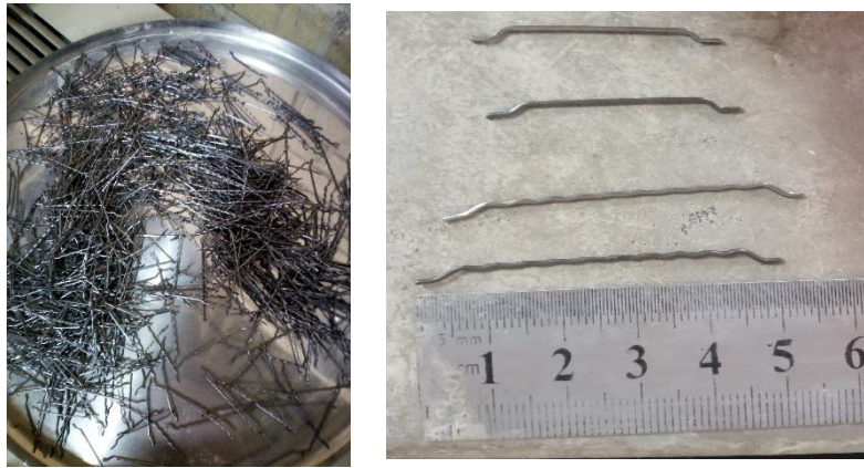
Figure 2. Two 3 and 5 cm lengths steel fibers
