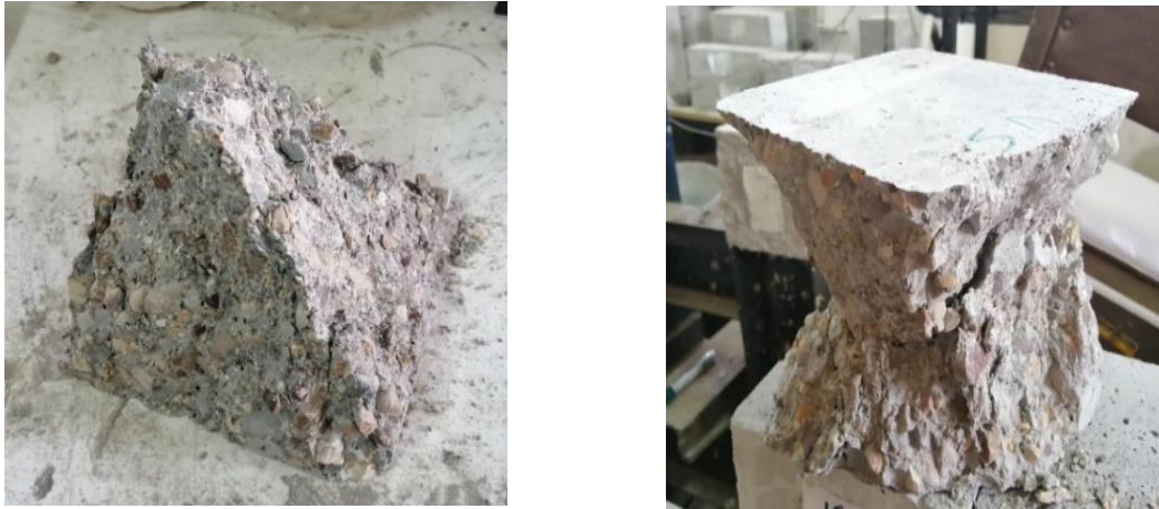
Figure 6. Simple cubic specimens after breaking
