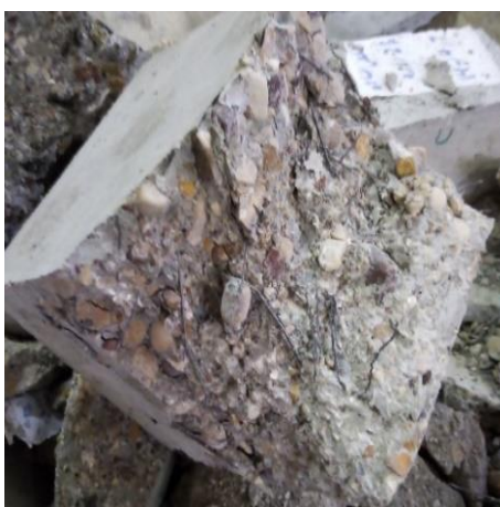
Figure 5. Cubic specimens containing steel fibers after breaking
