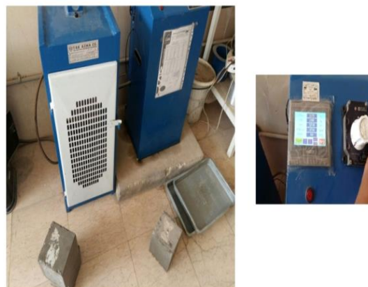
Figure 4. Determination of the compressive strength of concrete
