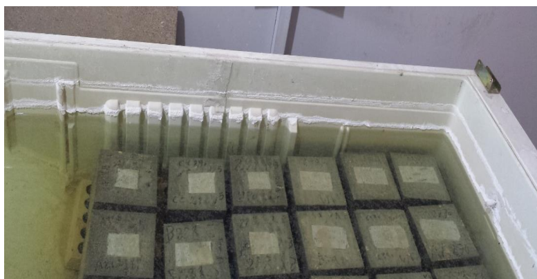
Figure 6. Sodium sulfate basin
