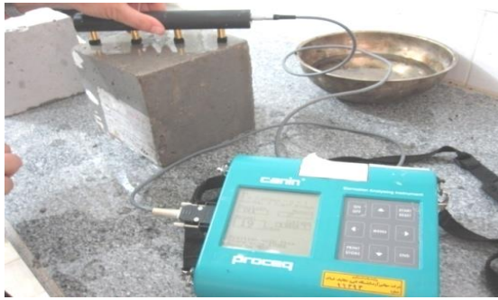
Figure 10. Apparatus of resisto-meter and the method used the electrical resistance of specimen
