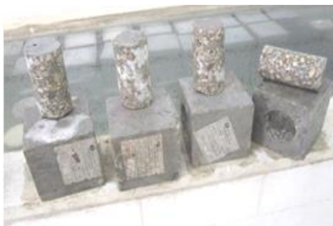
Figure 8. Core taken from cube specimens
