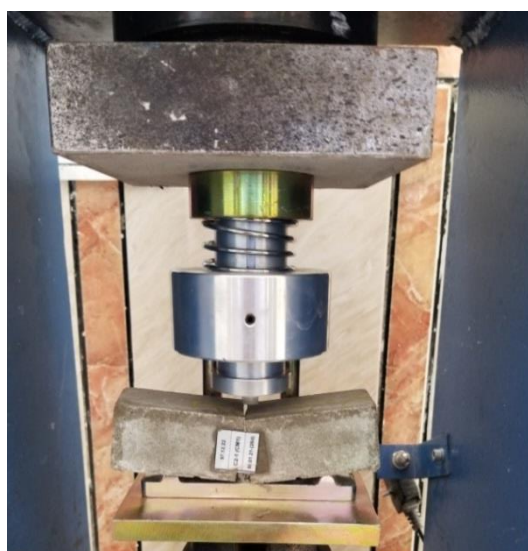
Figure 4. Flexural strength test setup for concrete specimens
