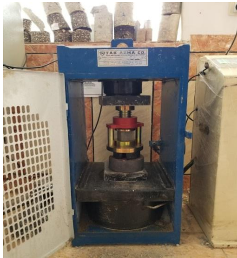
Figure 3. compression tests on 50mm cube
