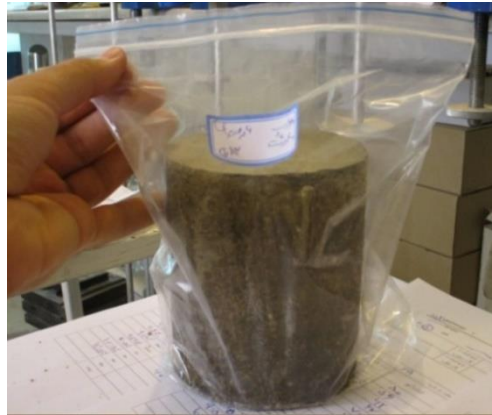
Figure 4. Sample cure in plastic bag.
