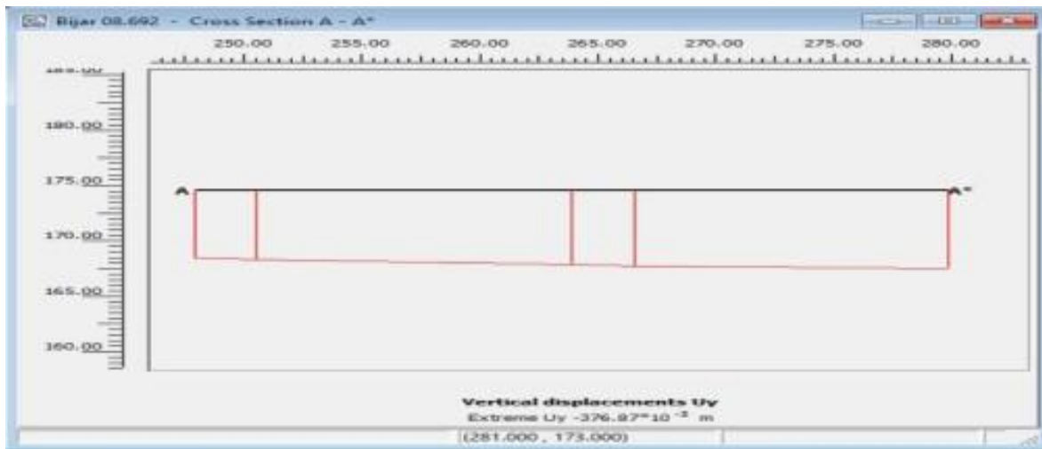
Figure 24. Changes in settlement at the end of construction by Plaxis at level of 175 m
